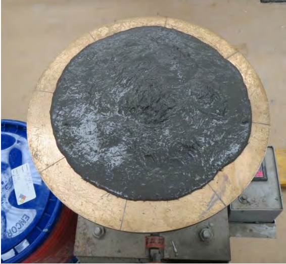
Figure 4. Photo. Nonthixotropic formulation.
