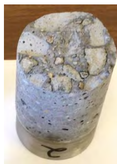
B. Mode 2: Bond failure at the interface.
