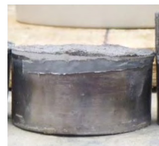
D. Mode 4: Failure in the disc adhesive.
