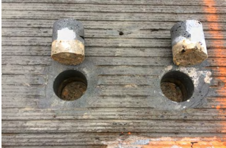
Figure 28. Photo. Two test samples after failure in the substrate concrete.
