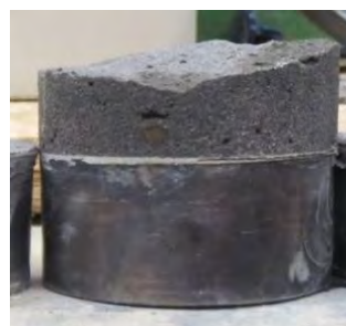
C. Mode 3: Failure in the bonded material.
