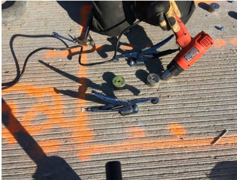
Figure 26. Photo. In-situ bond testing on the Laporte Road bridge.
