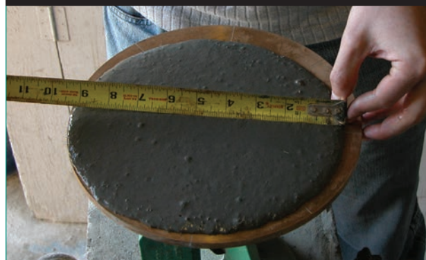
Figure 12. Photo. ASTM C1856 (C1437 mod.) flow test on UHPC. (25,9)
