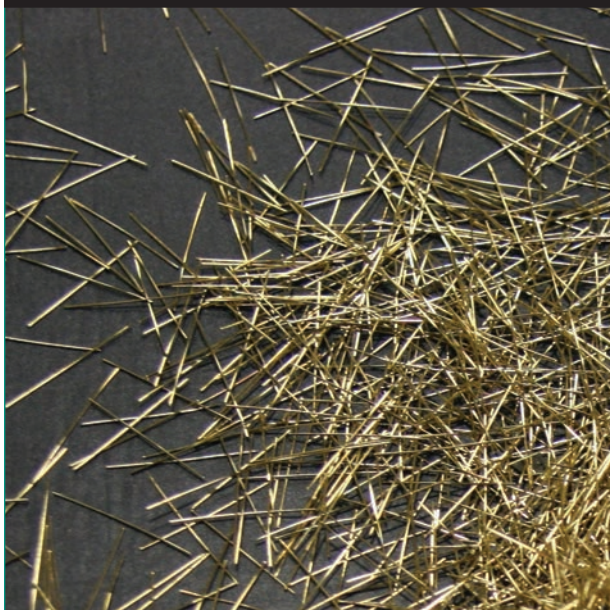
Figure 1. Photo. Commonly used steel fiber reinforcement. (25)
