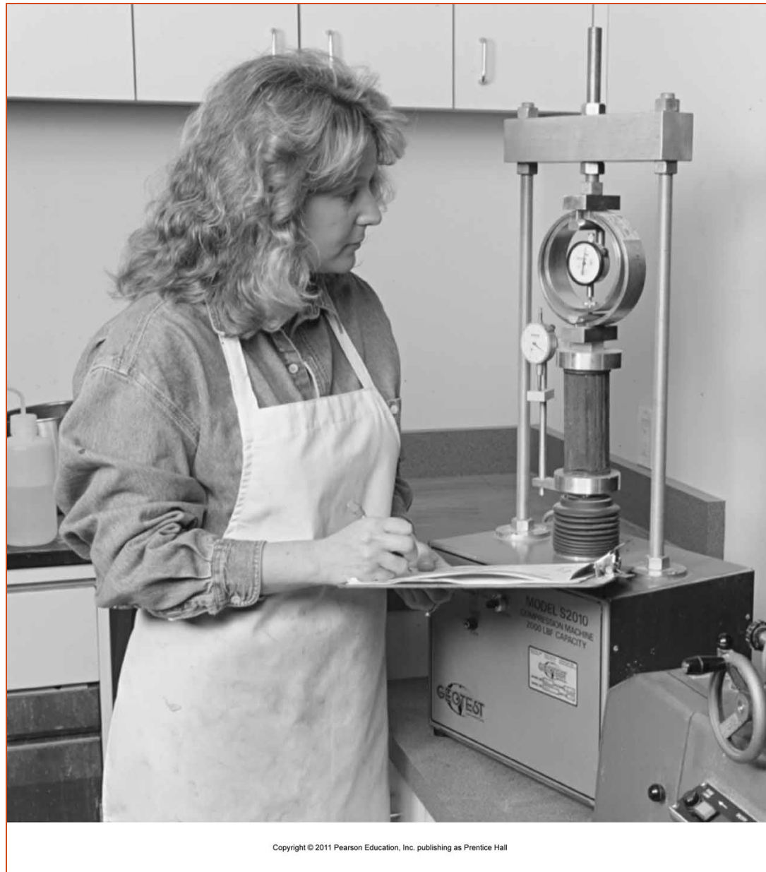
Figure Conducting an unconfined compression test.
