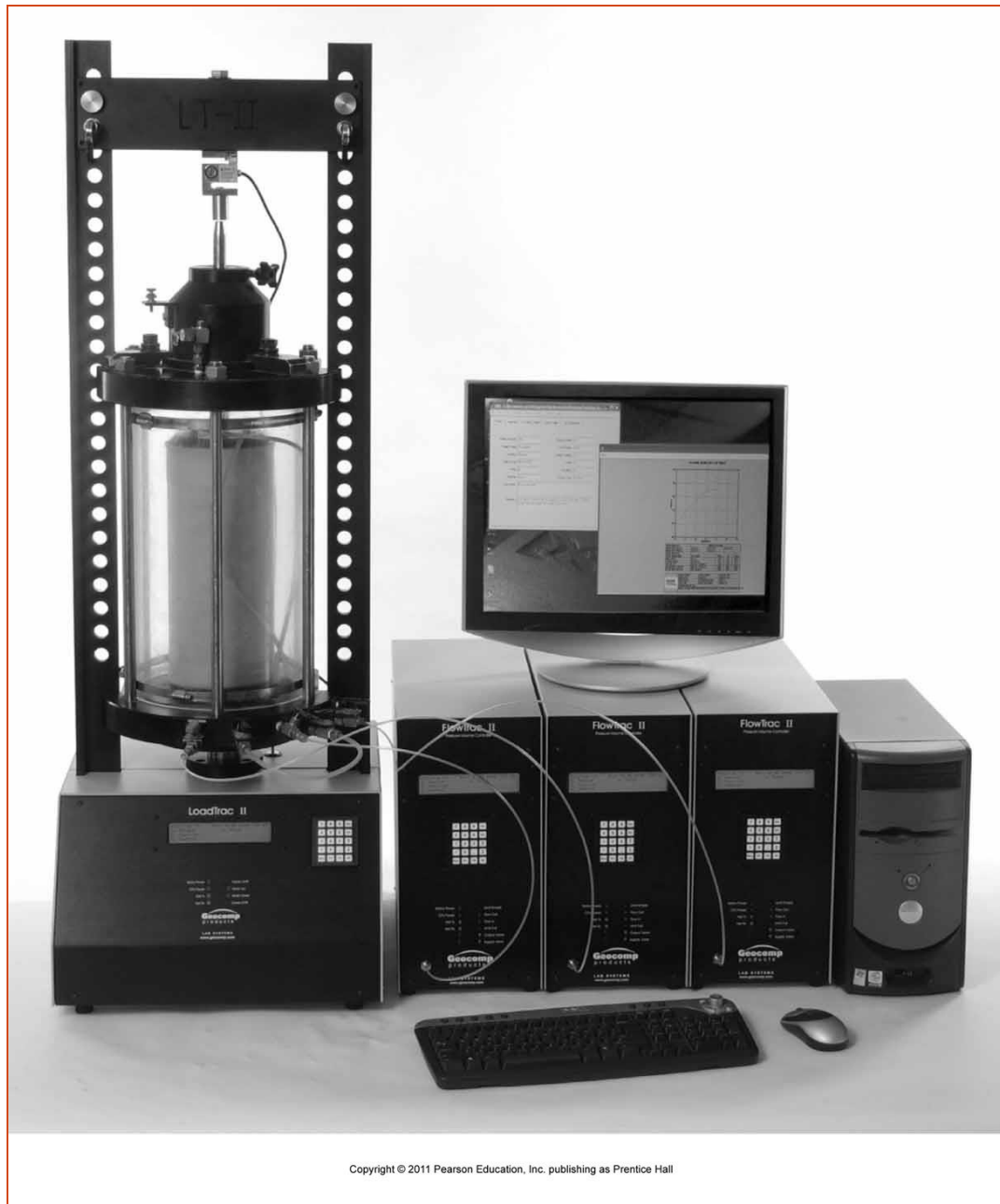
Figure Photograph of a typical triaxial test system. (Courtesy of Geocomp Corp.)
