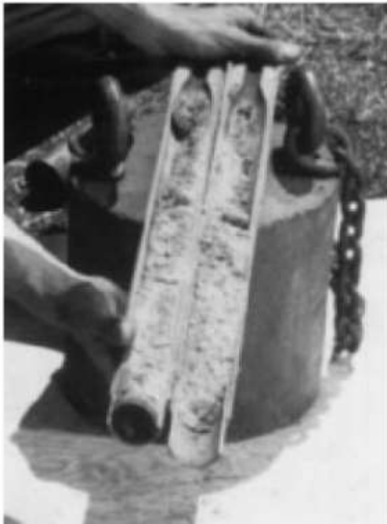
Figure 18.6 Split-spoon sampler, unassembled (Courtesy of ELE International)
