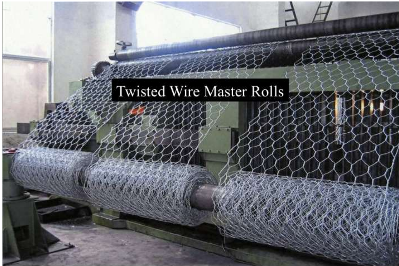
Twisted Wire Mesh Gabion Machine -Mesh is Produced in Rolls-
