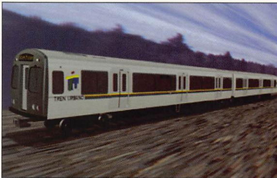
The Tren Urbano consists of specially designed stainless-steel vehicles configured in married pairs.
