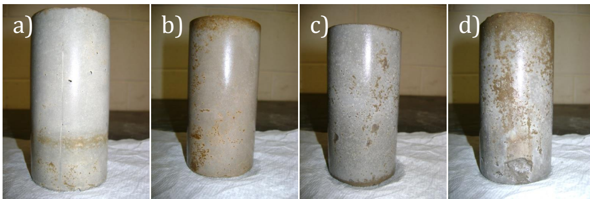
Figure 21. Cementitious pastes exposed to sulfuric acid for 7 days: a) 0%FA/B and 0% ENP/B, b) 0%FA/B and 3% ENP/B, c) 40%FA/B and 0% ENP/B, and d) 40%FA/B and 3% ENP/B.
