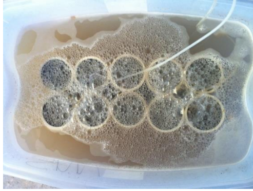
Figure 8. Specimens (design C-2) in water reservoir loaded with activated sludge
