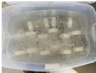
Figure 9. PCPC specimens (C-2 design) in reservoir with 0.1% H 2 O 2 solution
