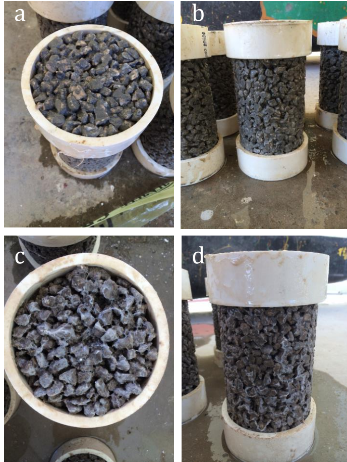
Figure 55. PCPC specimens after second clogging a)top view of C-2 PCPC, b) side view of C-2 PCPC, c) top view of optimum PCPC and d) side view of optimum PCPC
