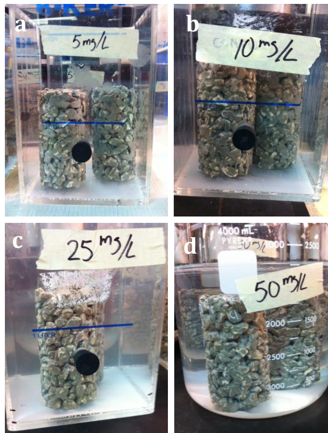
Figure 53. PCPC specimens after 72 hours exposed to a) 5mg/L, b) 10 mg/L, c)25 mg/L and d) 50 mg/L initial phosphate concentration
