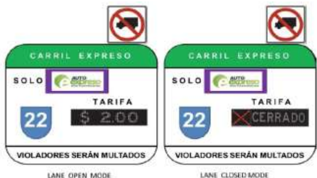
Figure 8: VMS Signs placed upstream of DTL entrance
