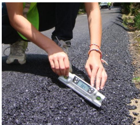
Figure 7. Slope measurement of 38.5 at PR-184, Patillas, PR
