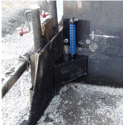
Figure 2. Safety Edge Shoe-TransTech: Shoulder Wedge Maker
