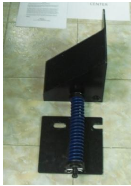
Figure 4. TransTech Shoulder Wedge Maker
